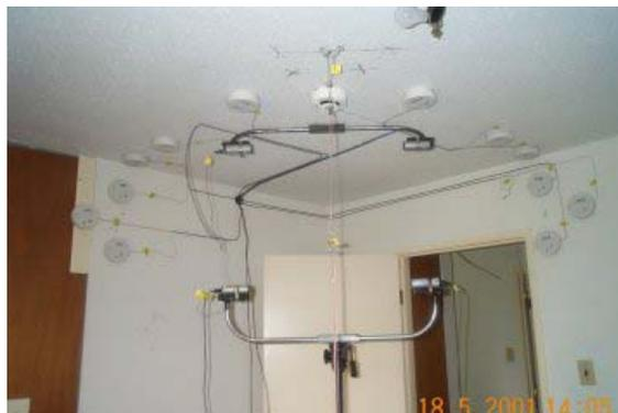
*Figure 1. Smoke-alarms installed in a bedroom.*
